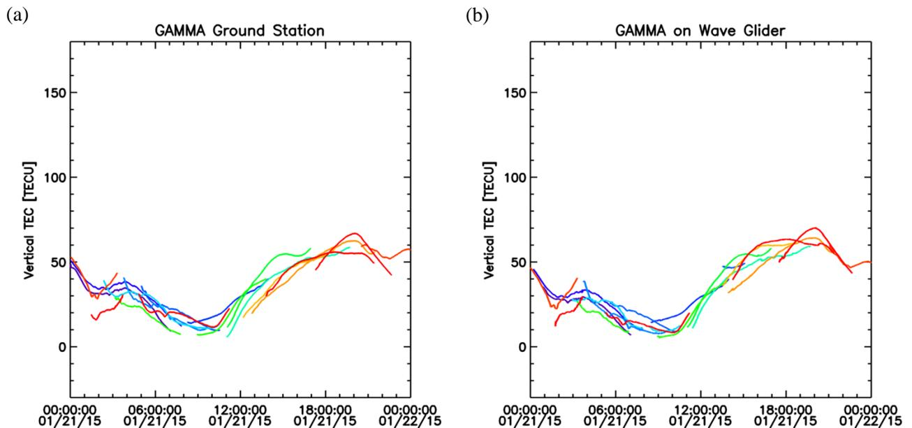
Figure 6. (a) VTEC from a GAMMA GPS receiver located at Lima, Peru (12 miles from the Wave Glider), (b) VTEC from the GAMMA GPS receiver on the Wave Glider while deployed 11 miles off the coast of Lima.
