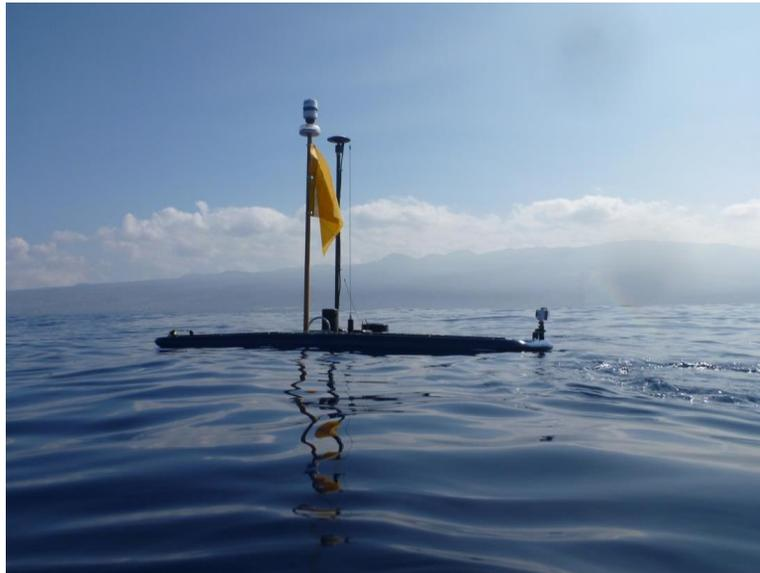
Figure 3. Wave Glider deployed off the coast of Lima, Peru on January 20, 2015. The GAMMA receiver is mounted under the solar panels in a Payload Dry Box. The GPS antenna is located on the top of the mast on the right.
