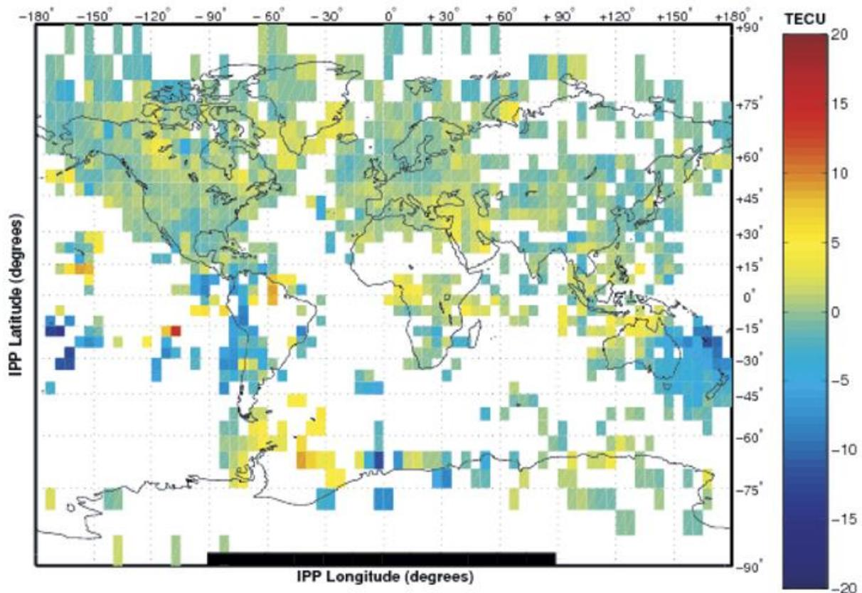
Figure 1. Global Map of the ionospheric Total Electron Content (TEC) showing measurements from ground-based dual-frequency GPS instruments. [Occhipinti et al., 2008].
