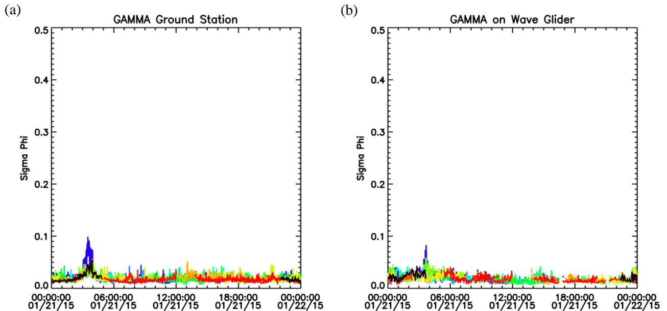
Figure 5. GAMMA  $\sigma_\phi$  from (a) a GAMMA receiver on shore in Lima, Peru; (b) the Wave Glider deployed 11 miles off the coast of Lima for a small scintillation event on January 21, 2015.
