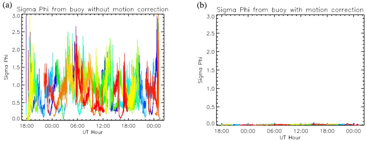
Figure 4. (a) Calculated phase scintillation index ( $\sigma_\phi$ ) without compensating for antenna motion on the Wave Glider. Note that strong ionospheric scintillations are often associated with a  $\sigma_\phi$  of around 0.8 cycles; (b) Same as (a) but now compensating for antenna motion.
