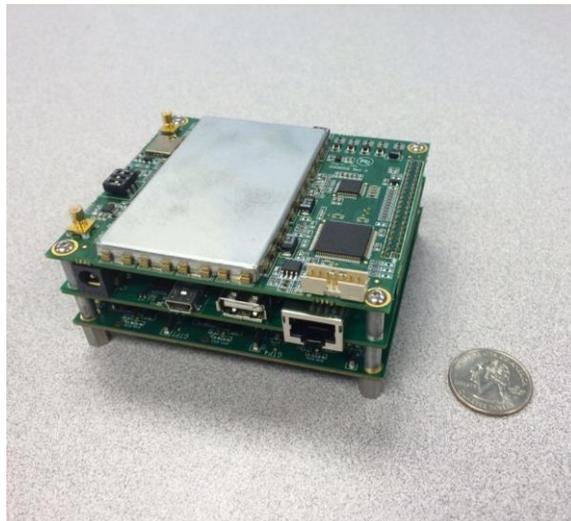
Figure 2. OEM version of the GAMMA GPS receiver showing the RF Front End (top board), the interface board (middle board), and the DSP board (bottom).
