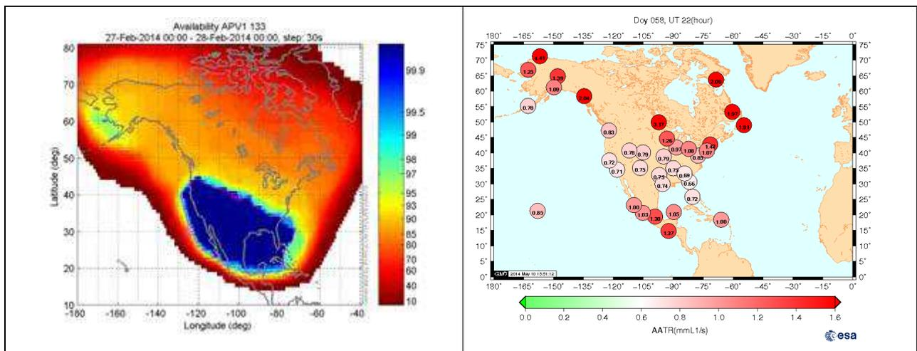
Figure 4. WAAS APV-1 availability (top) and AATR index computed for WAAS Reference Stations on the same day (27/02/2014) at hour 22-23 UT.
