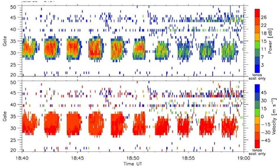
**Figure 2.** CUTLASS backscatter power, Doppler velocity, versus slant range in the heating region over EISCAT during one minute on (e. g. 18:44-18:45) and one minute off (e. g. 18:45-18:46) duty cycle during 18:40-19:00 UT on July 3, 2012.
