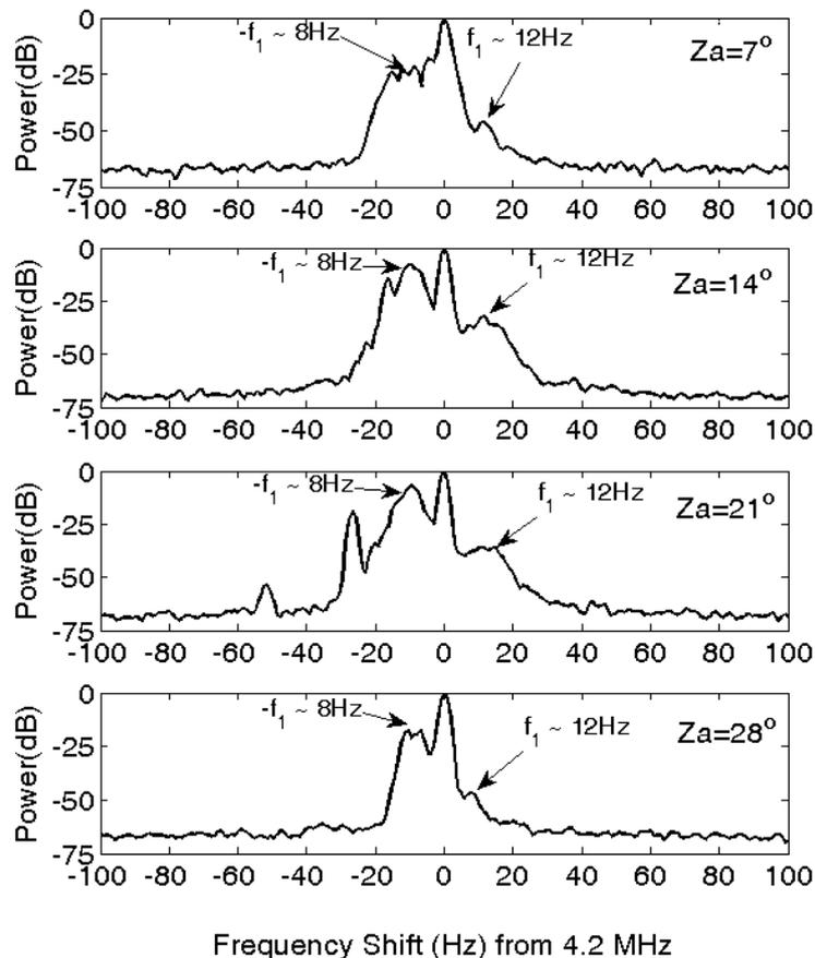
**Figure 3.** Measured frequency spectra of radio emissions from the HAARP at  $4.2\text{MHz}$  relatively close to  $3f_{ce}$  for different heater beam angles  $14^\circ$  (for the magnetic zenith) during 04:15-04:60 UT on July 22, 2010.
