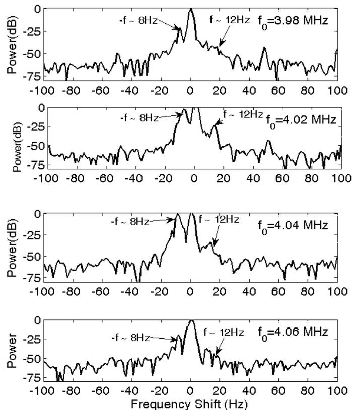
**Figure 1.** Measured frequency spectra of radio emissions from the EISCAT transmitter near  $3f_{ce}$  for the magnetic zenith pumping during 19:20 -19:32 UT on July 3, 2012
