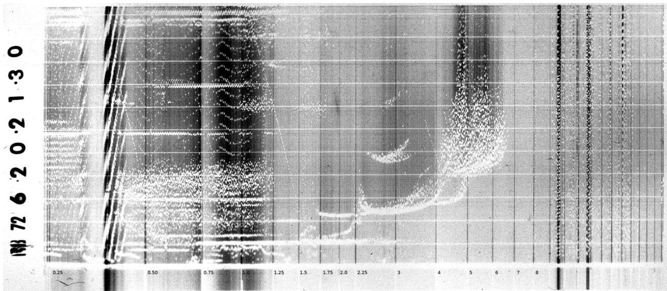
**Figure 5.** Resolute Bay ionogram taken just before the ISIS-2 pass. The ionogram frequency range was from 0.25-20 MHz and is indicated along the lower border of the image. Virtual height markers are at 100 km intervals.
