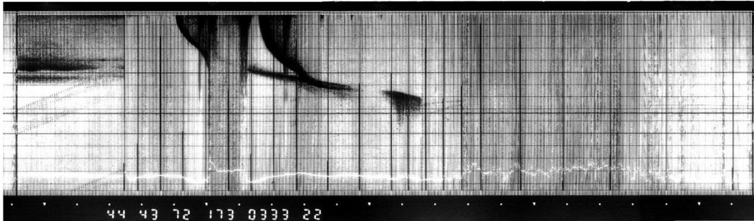
**Figure 2.** ISIS-2 full sounding sweep for 1972 day 173, starting at 03:33:22 UT. The 1.95 MHz fixed frequency sounding can be seen on the left, followed by the swept-frequency ionogram covering 0.1-20 MHz.
