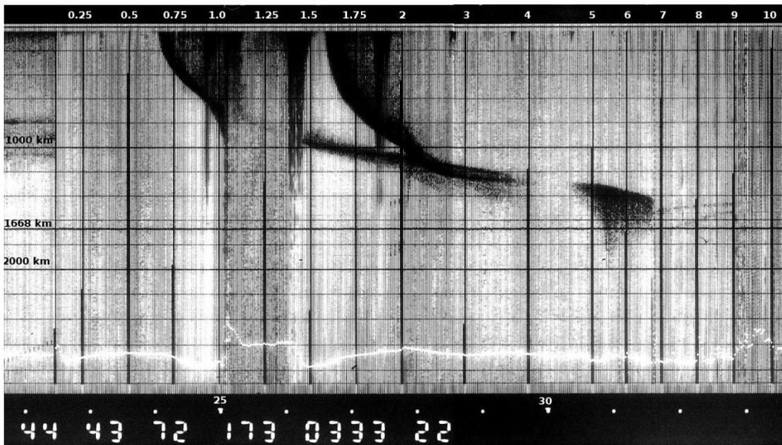
**Figure 3.** Enlarged section of Figure 2 showing the F-region topside traces. The frequency scale (MHz) is noted along the top edge, and the virtual distance is noted on the left side. The time ticks for 25 and 30 seconds are also marked.
