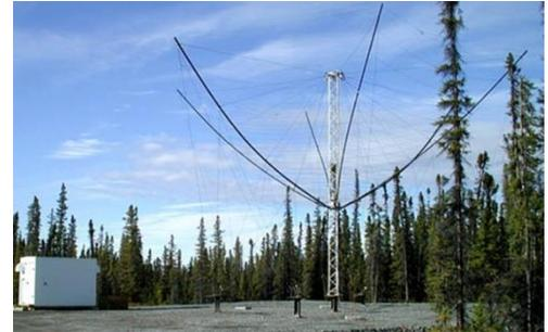
Figure 6 HF High Angle Receive Array
