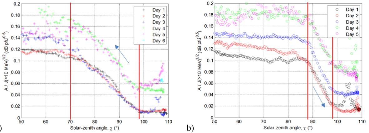
**Figure 4.** Ratio of absorption (dB) at the Fort Churchill riometer to the square root of  $> 10$  MeV proton flux for the SPE commencing 21 April 2002 as a function of solar-zenith angle. a) sunrise, b) sunset. The arrows indicate the change in  $\chi$  with time.
