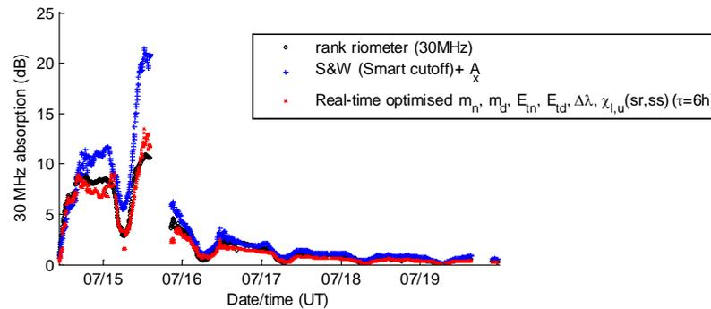
**Figure 7.** S&W (DRAP) predictions of absorption during the July 2000 SPE (blue '+') at the Rankin Inlet riometer (black  $\diamond$ ) and real-time-optimised  $m_n$ ,  $m_d$ ,  $E_{tn}$ ,  $\Delta \lambda$  (using all riometers)  $\tau = 6$  h.
