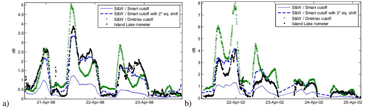
**Figure 2.** 30 MHz absorption at the Island Lake riometer during SPEs in a) April 1998 and b) April 2002 compared with predictions of S&W model (which uses the Smart cutoff model), S&W with a 2° equatorward shift of the Smart cutoff, and S&W with CL defined by (*Dmitriev et al.*, 2010).
