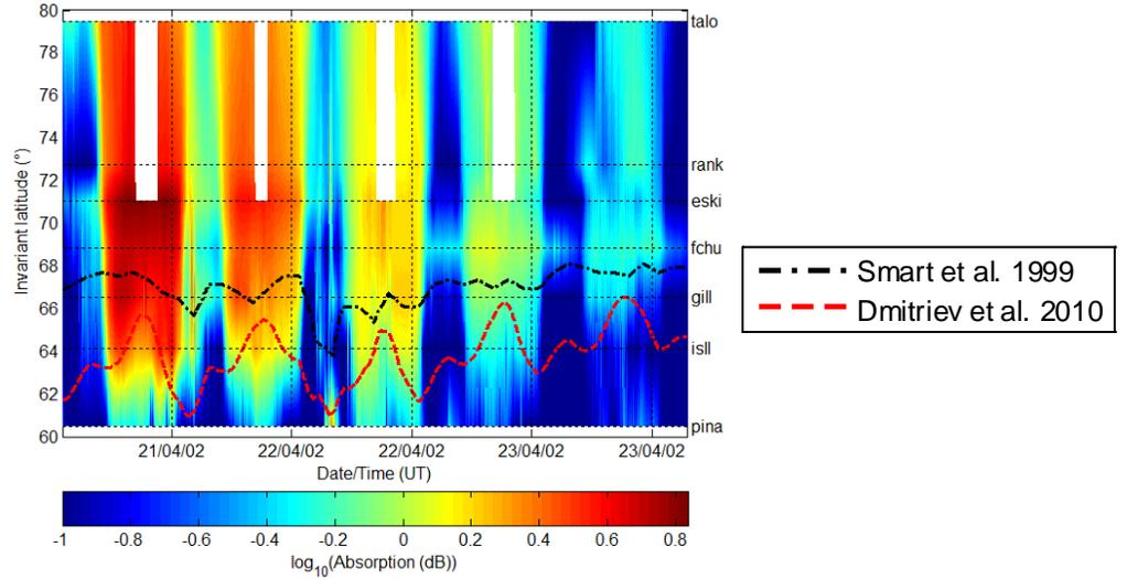
**Figure 1.** Two models of the cutoff latitude of 10 MeV protons (dashed lines) for the SPE of April 2002. Colours represent 30 MHz Cosmic Noise Absorption measured on seven riometers near the 94°W meridian, interpolated linearly in invariant latitude.
