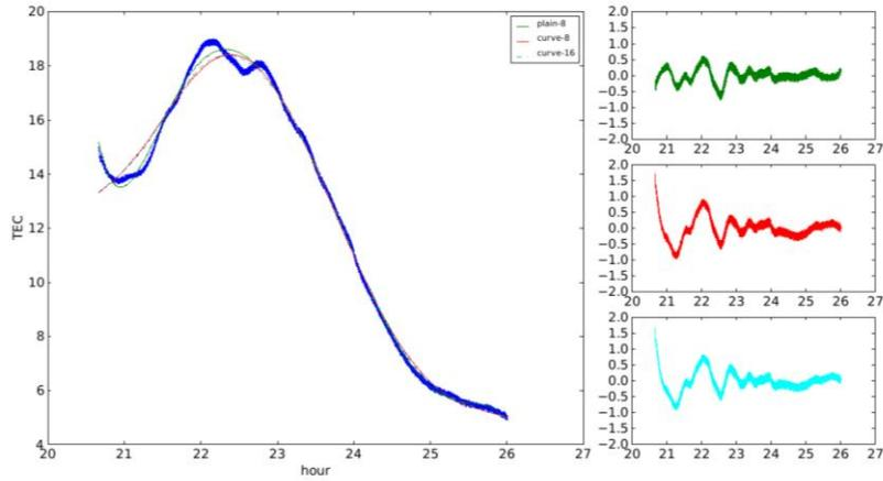
**Figure 7:** A typical TEC time series (dark blue) with three polynomial fittings. The green is 8th order, which over fits; the cyan is 16th order, and accurately preserves oscillatory behavior; the red is our Bayesian fit to the 8th order.
