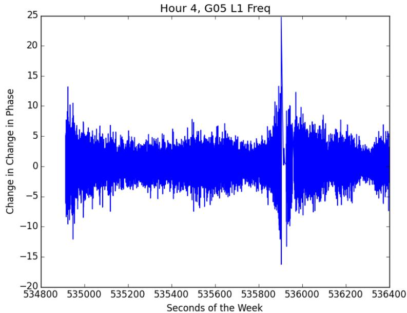
**Figure 2:** The double differential of a GPS time series, highlighting a dropout
